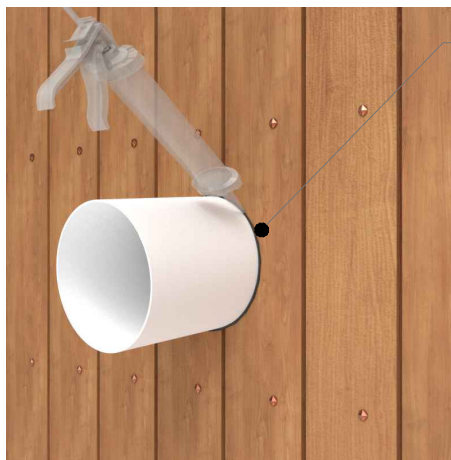
Continuous weather seal around pipe
