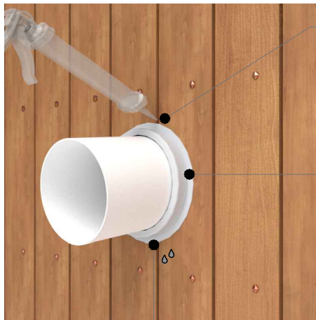
No sealant to drain
